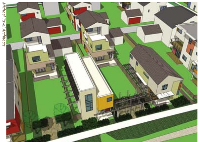
The Checkerboard Blocks section of the site plan includes single-family units spaced in a checkerboard pattern to allow solar access for neighboring units.
