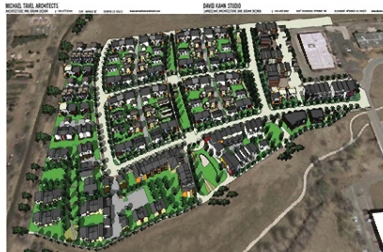
The community site plan for GEOS staggers homes into a checkerboard that allows each to gain some winter solar energy.
